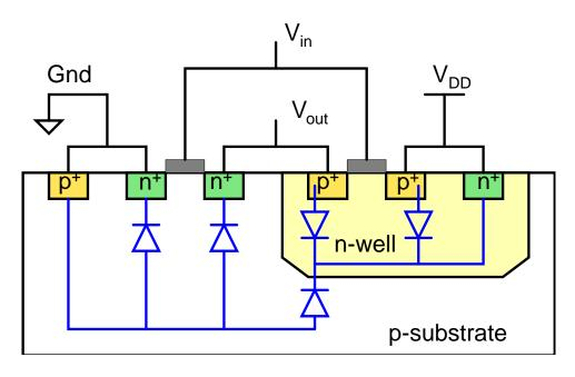
PN junction reverse bias leakage current
