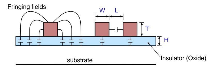
In addition, a conductor can exhibit capacitance to an adjacent conductor on the same layer
