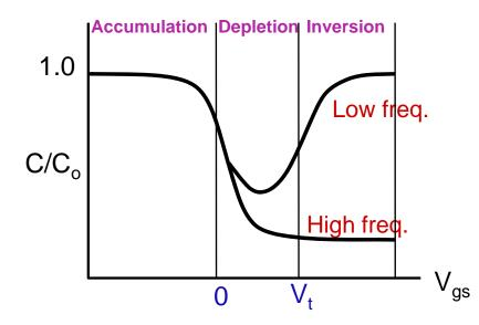
The minimum capacitance depends on the depth of the depletion region, which depends on the substrate doping density
