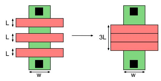
In general, the fall time t<sub>f</sub> is mt<sub>f</sub> (t<sub>f</sub>/m) for m ntransistors in series (parallel). Similarly the rise time t<sub>r</sub> for k p-transistors in series (parallel) is kt<sub>r</sub> (t<sub>r</sub>/k)
