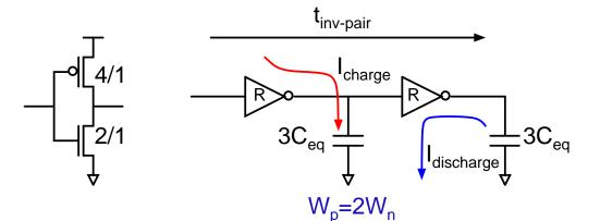
$$t_{inv-pair} = t_{fall} + t_{rise}$$
