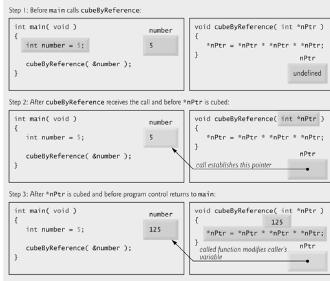
Fig. 7.9 | Analysis of a typical call-by-reference with a pointer argument.
