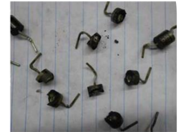
Overheated Bypass Diodes
