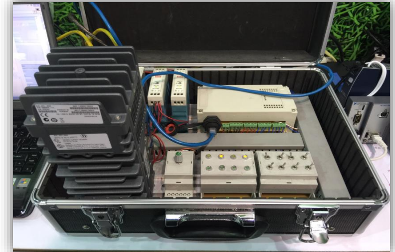
IEC61850/DNP3 Data Transformation Gateway
